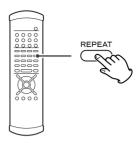
Use the REPEAT button to select the repeat mode for playback. Repeated presses of the REPEAT button cycle between the following options:
